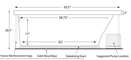
INSTALLATION: Height measurement is inclusive of wood and foam framing. All measurements are  $\pm$ 1/2" and are subject to change without notice. Drawing shows recommended pump location as well as approximate location of frame reinforcement legs. Please measure tub before building deck. Data herein supercedes all previous data prior to date shown below.
