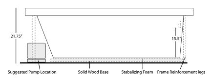
INSTALLATION: Height measurement is inclusive of wood and foam framing. All measurements are +/- 1/2" and are subject to change without notice. Drawing shows recommended pump location as well as approximate location of frame reinforcement legs. Please measure tub before building deck. Data herein supercedes all previous data prior to date shown below.
