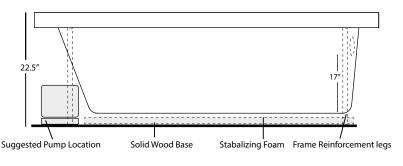
**INSTALLATION:** Height measurement is inclusive of wood and foam framing. All measurements are +/- 1/2" and are subject to change without notice. Drawing shows recommended pump location as well as approximate location of frame reinforcement legs. Please measure tub before building deck. Data herein supercedes all previous data prior to date shown below.
