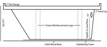
INSTALLATION: Height measurement is inclusive of wood and foam framing. All measurements are +/- and are subject to change without notice. Drawing shows recommended pump location as well as approximate location of frame reinforcement legs. Please measure tub before building deck. Data herein supercedes all previous data prior to date shown below.
