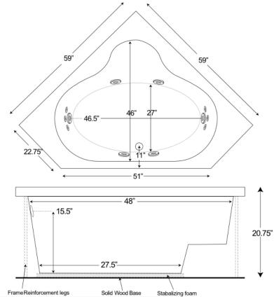
**INSTALLATION:** Heightmeasurement is inclusive of wood and foam framing. All measurements are +/- 1/2" and are subject to change without notice. Drawing showsrecommended pump location as well as approximate location of frame reinforcement legs. Pleasemeasure tub before building deck. Data herein supercedes all previous data prior to date shown below.
