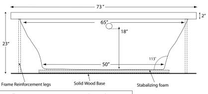
**INSTALLATION:** Height measurement is inclusive of wood and foam framing. All measurements are +/- 1/2" and are subject to change without notice. Drawing shows recommended pump location as well as approximate location of frame reinforcement legs. Please measure tub before building deck. Data herein supercedes all previous data prior to date shown below.
