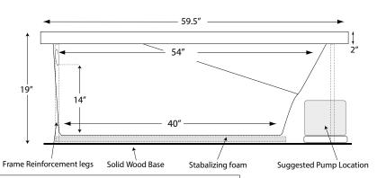
**INSTALLATION:** Height measurement is inclusive of wood and foam framing. All measurements are +/- 1/2" and are subject to change without notice. Drawing shows recommended pump location as well as approximate location of frame reinforcement legs. Please measure tub before building deck. Data herein supercedes all previous data prior to date shown below.
