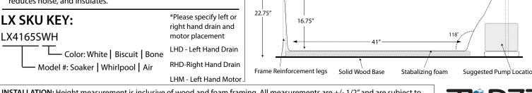
INSTALLATION: Height measurement is inclusive of wood and foam framing. All measurements are +/- 1/2" and are subject to change without notice. Drawing shows recommended pump location as well as approximate location of frame reinforcement legs. Please measure tub before building deck. Data herein supercedes all previous data prior to date shown below.
