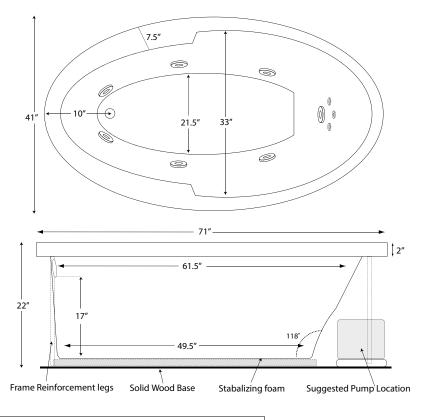
**INSTALLATION:** Height measurement is inclusive of wood and foam framing. All measurements are +/- 1/2" and are subject to change without notice. Drawing shows recommended pump location as well as approximate location of frame reinforcement legs. Please measure tub before building deck. Data herein supercedes all previous data prior to date shown below.
