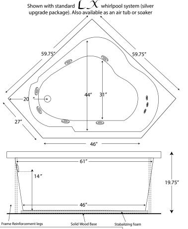
INSTALLATION: Height measurement is inclusive of wood and foam framing. All measurements are +/- 1/2" and are subject to change without notice. Drawing shows recommended pump location as well as approximate location of frame reinforcement legs. Please measure tub before building deck. Data herein supercedes all previous data prior to date shown below.
