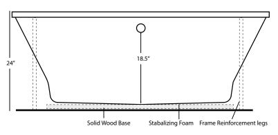
**INSTALLATION:** Height measurement is inclusive of wood and foam framing. All measurements are +/- 1/2" and are subject to change without notice. Drawing shows recommended pump location as well as approximate location of frame reinforcement legs. Please measure tub before building deck. Data herein supercedes all previous data prior to date shown below.
